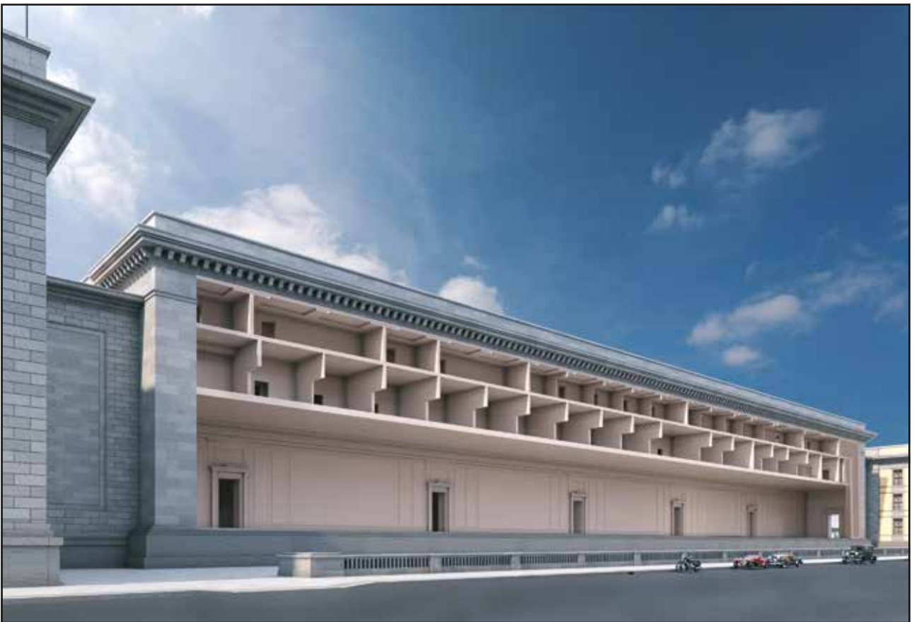
Fig. 59 This section drawing shows the actual ceiling heights of the rooms behind the facade
