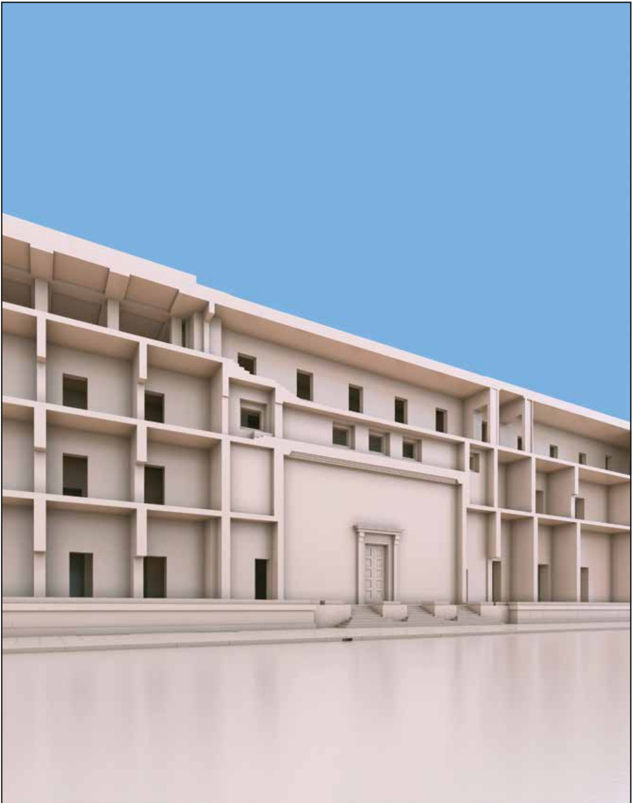
Fig. 59 Section through the corridors and rooms of the Presidential Chancellery on Voßstraße
