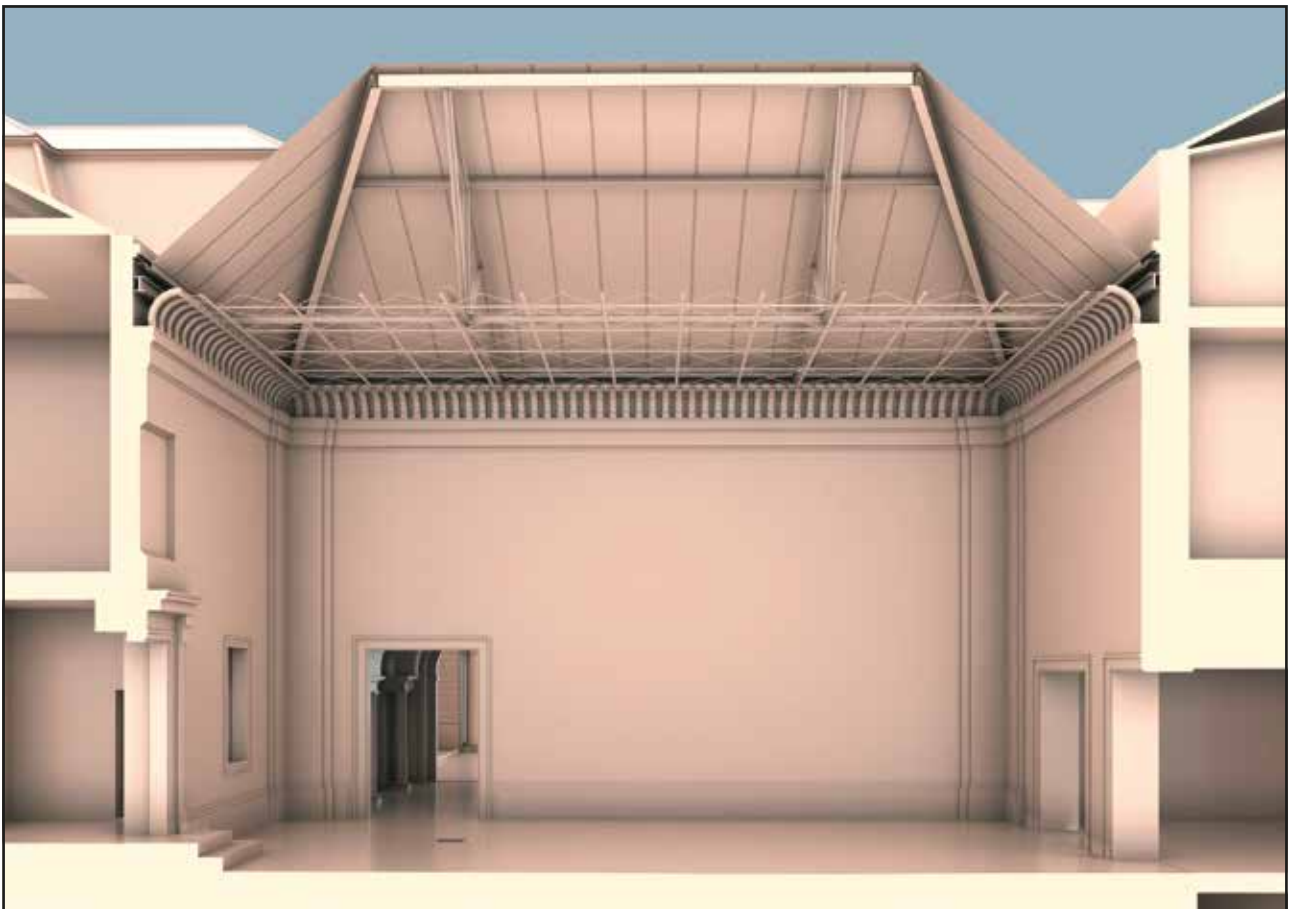
Fig. 24 Longitudinal cross-section through the Small Courtyard with a glass roof and attached ceiling.
