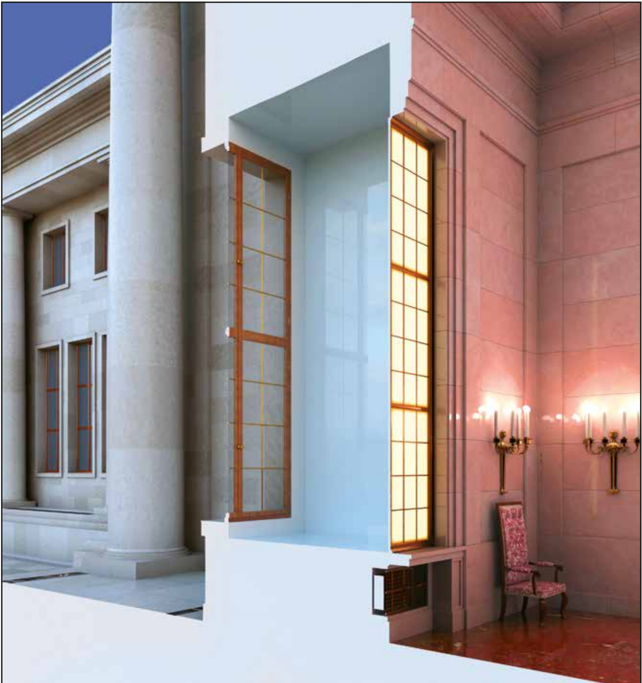
Fig. 55 Section through the window shaft - inside and outside windows were approx. 2.3m apart
