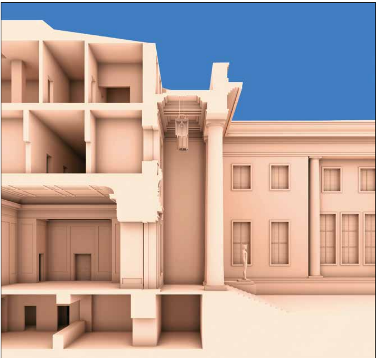
Fig. 65 The sectional view shows that the mezzanine windows of the portal belonged to small office rooms
